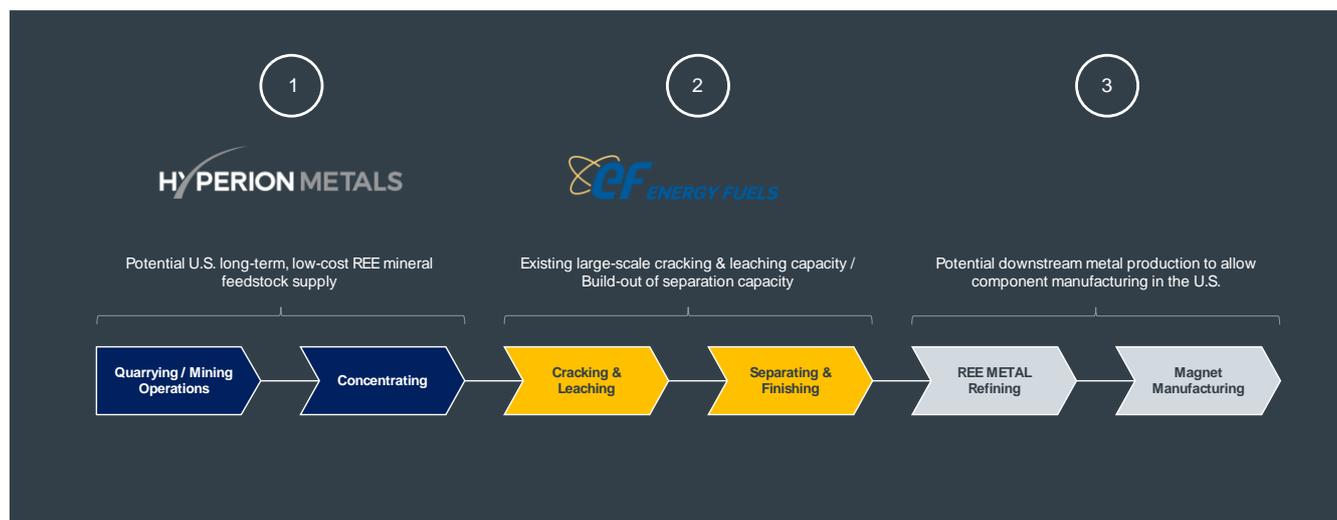
**Figure 1: Neodymium magnet supply chain and involvement by Hyperion & Energy Fuels**
